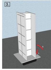
All fasteners hand-tighten only, do not overtighten!
